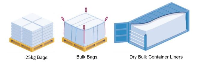
Figure 4: Types of plastic pellet packaging. Source: ITOPF
