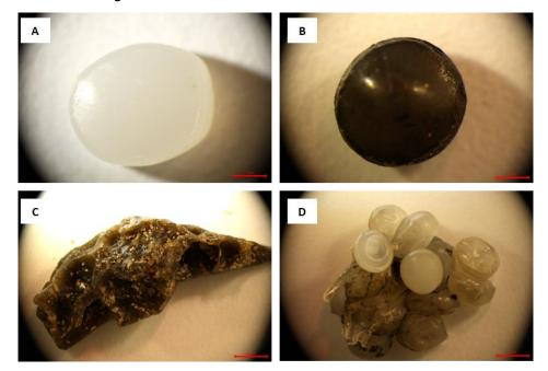
Figure 8: Morphological changes of plastic pellets following combustion during X-PRESS PEARL incident, Sri Lanka, 2021. A) original pellet; B) discoloured pellet; C) burnt plastic pellet fragment; D) fused pellets. Source: Cefas
