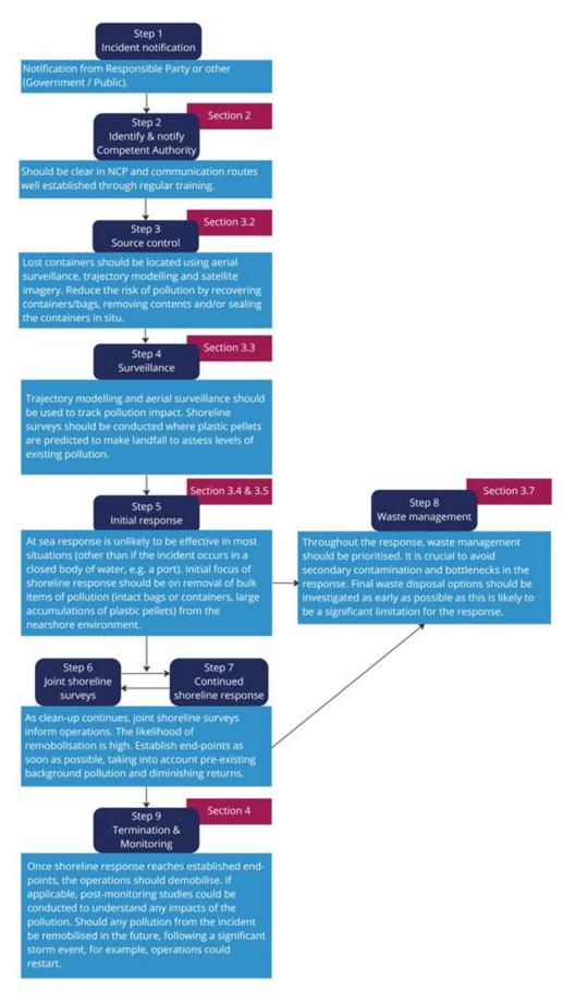
Figure 1: Flowchart to illustrate typical steps to take following a ship-source plastic pellet spill, with reference to sections of this document for further information.
