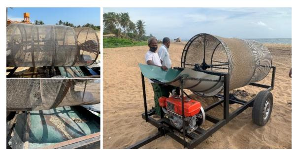
Figure 20: Mechanical trommels. Source: ITOPF.
