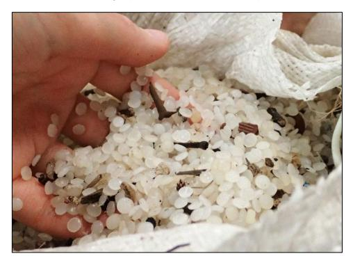
Figure 2: White plastic pellets. Source: ITOPF
