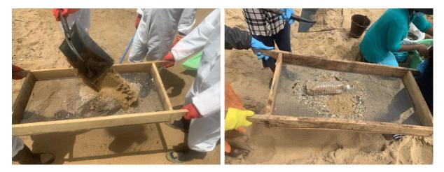
Figure 16: Single layer wooden sieve. Source: ITOPF
