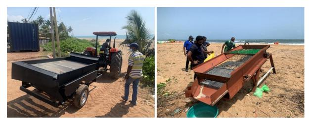
Figure 21: Mechanical table screeners. Source: ITOPF
