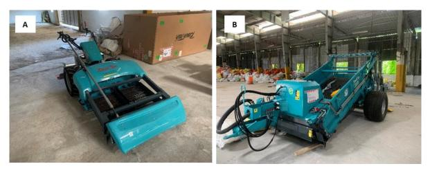
Figure 22: Different types of beach cleaners. A) walk-behind; B) tractor drawn. Source: ITOPF.
