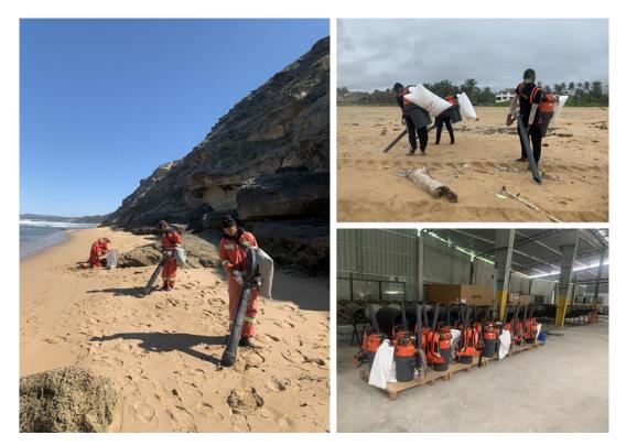
Figure 19: Vacuum recovery units. Source: ITOPF.
